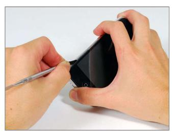
If necessary, insert the metal spudger in the same manner on the side of the iPhone and continue to pry up gently. Stop using the metal spudger once the display assembly is up enough that you can lift it up with your fingers.
