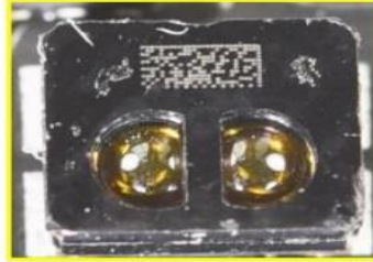
proximity sensor (mnf. unknown) 2.78 mm x 2.38 mm x 1.28 mm
