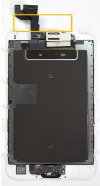
proximity sensor (mnf. unknown) 2.78 mm x 2.38 mm x 1.28 mm
